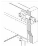
Front Pedestal Lock System Can be fitted into top drawer, cross rail or pen tray.
